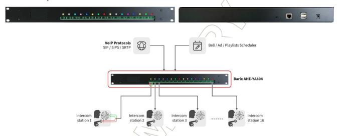
The Annuncicom AHE-YA404 is a powerful all-in-one Analog Head End solution designed to modernize legacy 2- or 4-wire intercom and paging systems—without the need to replace existing cabling or call stations. With integrated **VoIP SIP support** and onboard amplification, the AHE-YA404 enables seamless paging and intercom functionality from standard SIP phones to **up to 16 individual 2 or 4 wire intercom panels**.
