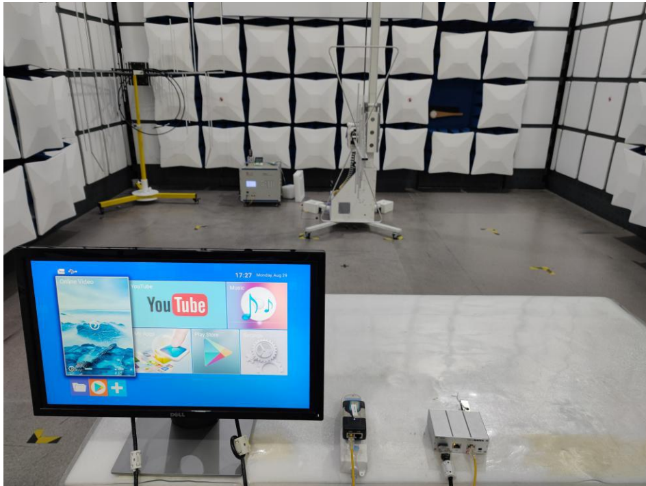
EUT Photo RE(POE power supply)
