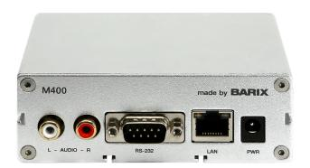
The BARIX M400 SIP Opus Encoder/Decoder allows to establish a link between devices using standard SIP protocol in peer-to-peer mode or through a SIP server. The unit provides an Opus encoded stereo link with line audio input or output. It also supports USB sound devices. Other common VoIP codecs including G.711 and G.722 are supported. This makes the BARIX M400 SIP Opus Encoder/Decoder the ideal product for high quality audio distribution or contribution in a SIP based environment.
