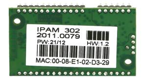
For hardware integration a development specification with schematic, pinout and suggestions for the layout of a custom carrier PCB is available. Barix Annuncicom60 and Instreamer are based on this module.
