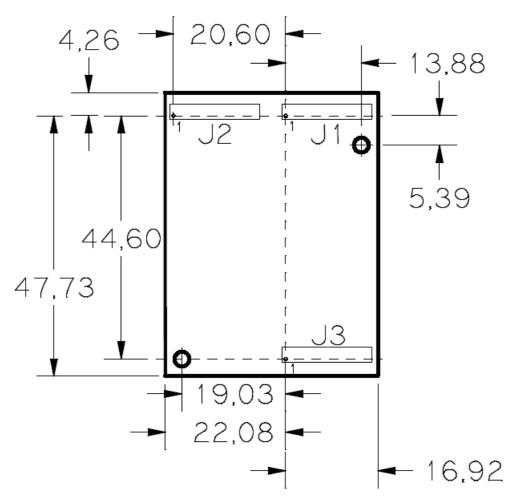
The above drawing shows the component side which faces down onto the carrier PCB.
