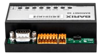
The Barionet 50 is a low cost, flexible and multiprotocol capable I/O device server which bridges the physical world of sensors and activators with IP Automation and IT management systems.
