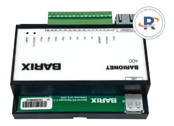
Barionet 400 Syn-Apps is a PoE powered I/O device server which is certified for the Syn-Apps' Revolution mass notification system. The device features four digital inputs and four relays. Extension
