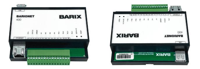
Barix Barionet 400 InformaCast is a PoE powered I/O device server which is certified for Singlewire's mass notification system InformaCast adopting the M2M capability. The device features four digital inputs and four relays. Extension of the functionality via the USB port
