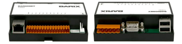
Barionet 1100 is a device server, based on Linux/Lede/OpenWRT. The device features a wide range of interfaces such as two USB, WiFi, RS322 serial port, analog and digital I/Os, Relays and Dallas 1-wire support. It is IPv4 or IPv6 capable. Supporting SNMP, Modbus and universal ASCII protocols, the Barionet device can be easily integrated into 3rd party management systems. Barix Products are developed in Switzerland and manufactured in the EU.
