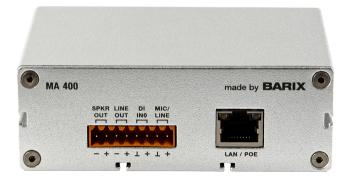
The BARIX MA400 SIP Opus Codec allows to establish a link between devices using standard SIP protocol in peer-to-peer mode or through a SIP server. The unit provides an Opus encoded bi-directional mono link with microphone or line input and line and speaker output. Other common VoIP codecs including G.711 and G.722 are supported. This makes the BARIX MA400 SIP Opus Codec the ideal product for audio distribution or contribution and intercom in a SIP based environment.
