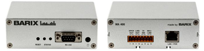
The BARIX MA400 SIP Opus Codec allows to establish a link between devices using standard SIP protocol in peer-to-peer mode or through a SIP server. The unit provides an Opus encoded bi-directional mono link with microphone or line input and line and speaker output. Other common VoIP codecs including G.711 and G.722 are supported. This makes the BARIX MA400 SIP Opus Codec the ideal product for audio distribution or contribution and intercom in a SIP based environment.
