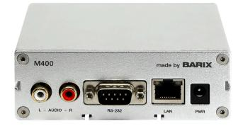
The BARIX M400 SIP Opus Encoder/Decoder allows to establish a link between devices using standard SIP protocol in peer-to-peer mode or through a SIP server. The unit provides an Opus encoded stereo link with line audio input or output. It also supports USB sound devices. Other common VoIP codecs including G.711 and G.722 are supported. This makes the BARIX M400 SIP Opus Encoder/Decoder the ideal product for high quality audio distribution or contribution in a SIP based environment.
