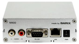
The Instreamer ICE encodes analog audio into MP3 or AAC+ for streaming to an Icecast internet radio streaming service in the cloud. The Instreamer ICE also has an Icecast server built in and is able to feed up to 100 web radio listeners directly without the requirement to subscribe to an internet radio service provider.
