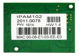
The Barix IP AUDIO MODULE 102 is a versatile network audio module that encodes and decodes PCM, G.711, G. 722 and MPEG audio. The IPAM 101 model is intended for OEM applications where G.722 and MP3 encoding is not required. Both models enable manufacturers of traditional audio devices to add network capabilities to their products.
