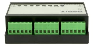
Barix Barionet R6 is a DIN-rail mountable relay module for commercial control, power switching and home automation applications. Using the industry standard Modbus protocol over 2-wire RS-485 the device can be controlled from any Modbus capable master. Each relay has three connections (common, normally closed and normally open) available at screw terminal blocks supporting wires from AWG 26 / 0.15 mm2 up to AWG 14 / 2.5 mm2.
