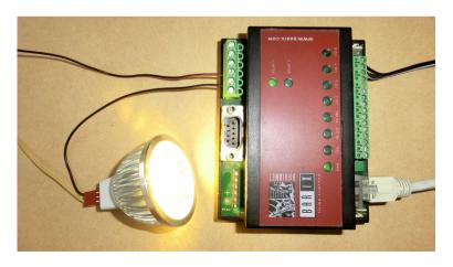
The wiring to connect your electrical device to the Barionet relay is pretty simple. Your electrical device has typically two wires (+ and -). Simple spoken you have to cut through one of these two wires in the middle and connect these two ends to the relay, one end to Common (pin 4 of J3) and the other end to NO (pin 5 of J3) or NC. But before you do that make sure your complete equipment is not powered during the installation!
