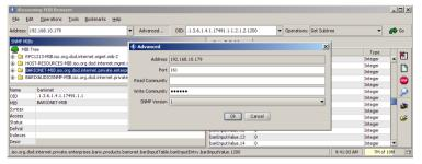
To write to the Barionet's SNMP register select one of the Barionet input (IO) registers and select the "Set" option.
