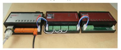
When you will connect more than one extension unit then connect it to the previous extension unit also over an additional 4-pin extension cable. The 4-pin cable provides power and also the RS485 connection to the extensions.
