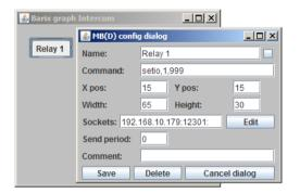
In the left picture a new direct Message button will be created which sends the command "setio,1,999" when pressed. This command will toggle the Barionet relay 1 to reverse state as soon the command is received.
