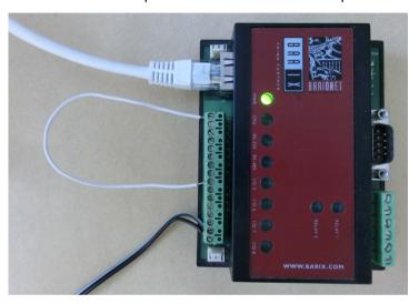
On the Barionet100 connect e.g. Pin1 and Pin9 of the J6 connector (see picture above).
