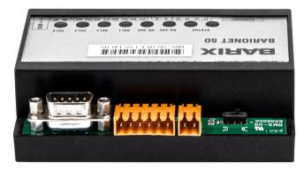
The Barionet 50 is a low cost, flexible and multiprotocol capable I/O device server which bridges the physical world of sensors and activators with IP Automation and IT management systems.
