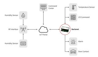
Barionet 400 is a fully programmable I/O device server of Barix, based on Linux/Lede/OpenWRT. The device features most common IO interfaces such as USB, digital Inputs and Relays. It is IPv4 or IPv6 capable. Supporting multiple communication protocols, the Barionet device can be used in different applications such as automation, building control, public transport and many more. Barix Products are developed in Switzerland and manufactured to the highest standards.
