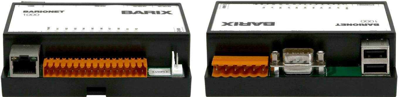
Barionet 1000 is a device server, based on Linux/Lede/OpenWRT. The device features a wide range of interfaces such as two USB, WiFi, RS322 serial port, analog and digital I/Os, Relays and Dallas 1-wire support. It is IPv4 or IPv6 capable. Supporting SNMP, Modbus and universal ASCII protocols, the Barionet device can be easily integrated into 3rd party management systems. Barix Products are developed in Switzerland and manufactured in the EU.
