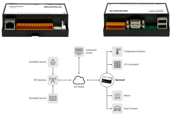
Barionet 1000 is a device server, based on Linux/Lede/OpenWRT. The device features a wide range of interfaces such as two USB, WiFi, RS322 serial port, analog and digital I/Os, Relays and Dallas 1-wire support. It is IPv4 or IPv6 capable. Supporting SNMP, Modbus and universal ASCII protocols, the Barionet device can be easily integrated into 3rd party management systems. Barix Products are developed in Switzerland and manufactured in the EU.
