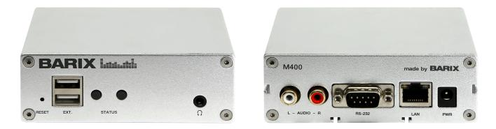
The AudioPoint 3.0 encodes analog audio and streams it with lowest latency to a free to download iOS or Android app. AudioPoint 3.0 allows to bring the audio of live events, live translation services or the audio of digital signage appliances or TV screen over a wireless router to many user's smartphones.
