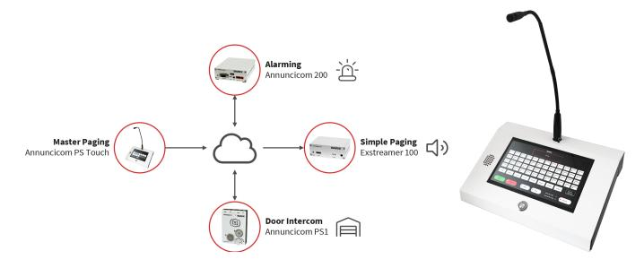
The Barix Paging Station Annuncicom PS Touch is a universal, TCP/IP connected intercom station for use in IP Intercom, Paging and VoIP applications. The PS Touch directly connects to the network via a 10/100Mbps connection, and is powered over the network interface (PoE, 802.3af standard).
