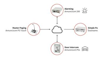
The Barix Paging Station Annuncicom PS Touch is a universal, TCP/IP connected intercom station for use in IP Intercom, Paging and VoIP applications. The PS Touch directly connects to the network via a 10/100Mbps connection, and is powered over the network interface (PoE, 802.3af standard).
