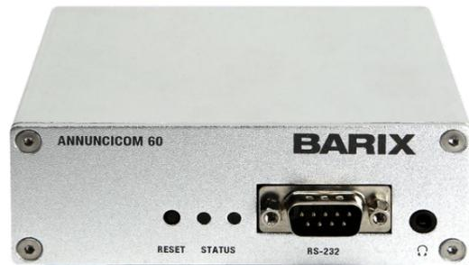
The Annunicom 60 is a generic IP Audio device designed to serve as a gateway between IP based VoIP, Paging, Intercom systems and traditional systems or call boxes, loudspeakers and microphones.
